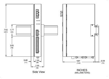
STR-100 and STR-100-IRIG-B front and side views with dimensions (DIN-rail mounting)
