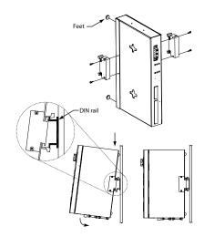
STR-100 and STR-100-IRIG-B mounting on standard DIN rail
