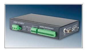
The Cyber Sciences' Satellite Time Reference STR-100/IRIG-B accepts a Global Positioning System (GPS) time signal from a Trimble Acutime 360 GPS smart antenna and outputs a precision time reference in unmodulated IRIG-B format.
