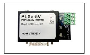
The Cyber Sciences Precision Timing Protocol (PTP) Legacy Interface (PLXe-5V) is a wiring adapter for the CyTime<sup>™</sup> Sequence of Events Recorder to output a legacy time protocol to other devices. The adapter fits the "Options" port (DB15 connector) of the SER-32e and facilitates wiring of 5V signals via a screw-type terminal, suitable for power equipment wiring.
