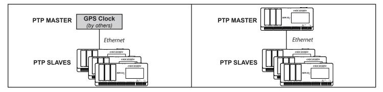
Figure 3-4. SER-32e as PTP slave(s) using PTP over Ethernet to sync with PTP master clock by others
