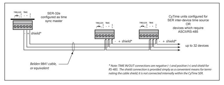
Figure 3-8 SER inter-device (RS-485) time sync input/output or ASCII/RS-485 time-sync output
