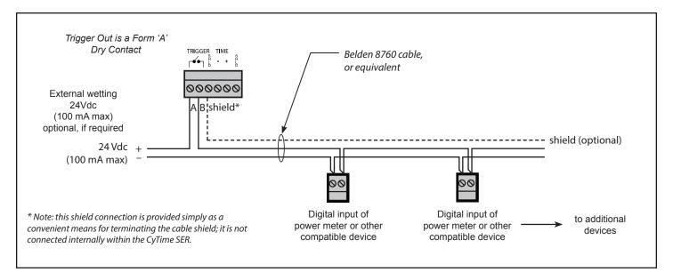
Figure 3-9. Trigger output connection to multiple devices
