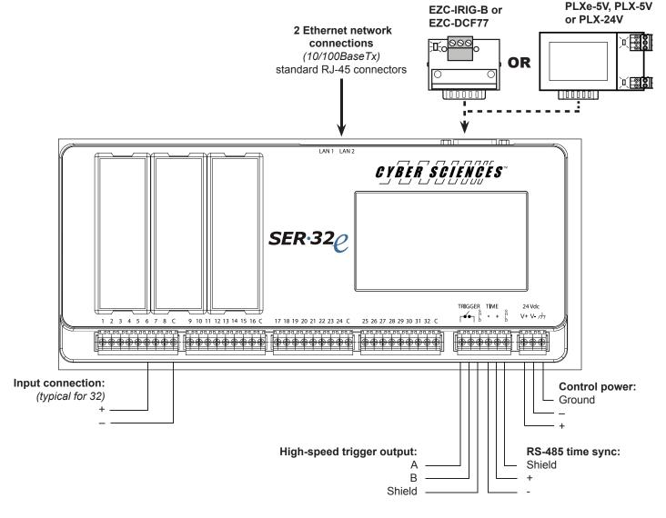
Figure 3-1. SER-32e wiring connections
