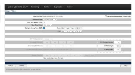
Figure 5-5. Time setup web page (with PTP time source setting shown)
