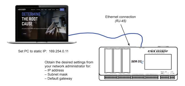
The SER has two (2) Ethernet ports (LAN1 / LAN2). Either port can be used, but only one can be connected at a time. If two ports are connected, only LAN 1 will be active.
