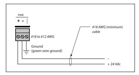
Figure 3-3. Control power connections
