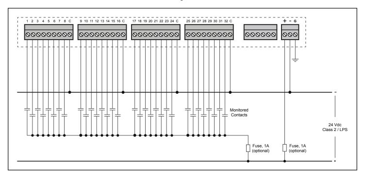
Figure 3-2. Digital input wiring connections (SER-32e)
