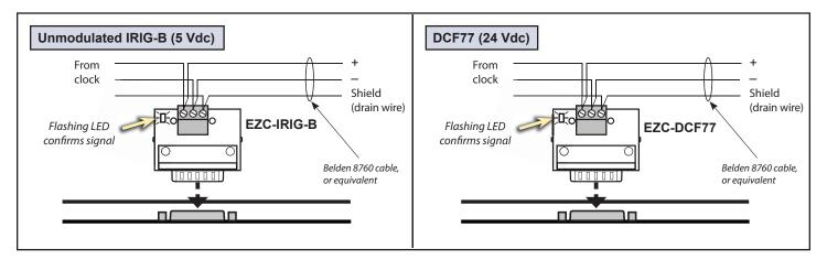
Figure 3-6. CyTime SER uses optional EZC-IRIG-B or EZC-DCF77 to accept time source of IRIG-B or DCF77, respectively
