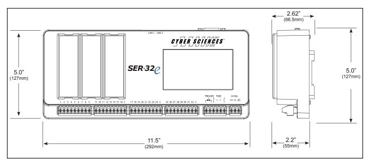
Figure 2-1. Front and side views, with dimensions—SER-32e
