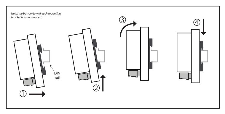
Figure 2-2. DIN-rail mounting (side views)
