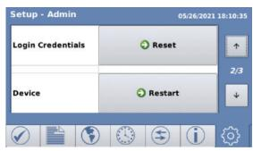
To change communications settings from the SER front panel, select the GEAR icon ((a)) and press the EDIT button (page 1/3):
